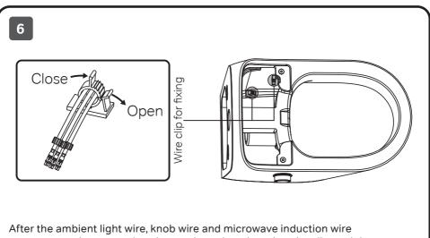
After the ambient light wire, knob wire and microwave induction wire are connected, arrange the wires and put them into the wire clip, and then press and hold the wire clip in the direction of closing indicated by the arrow. When you need to take out thewire, press the wire clip in the direction of opening indicated by the arrow.
