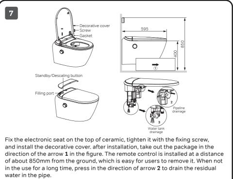
Before replacement or maintainence, pls pull down according to the arrow **3** direction below, and drain the residual water inside the wank first.
