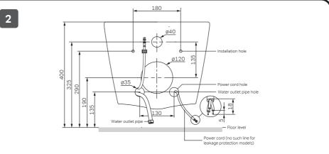
Put the toilet mat on the reserved position on the wall, direct the mounting hole of toilet mat to the fixed screw of the water tank frame, and then insert the mat, aligning with the flushing hole and sewage hole of the water tank, and pass the water outlet pipe through the water outlet hole, and the power cord passes through the power cord hole, exposed outside the wall.
