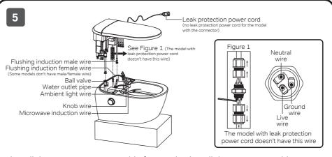
Install the power connector cable (no need to install the connector cable for the model with leakage protection plug), ambient light cable, knob cable, and microwave induction cable as shown in the figure. Note: When wiring, you need to disassemble the upper part of the waterproof plug, check whether the ground wire, neutral wire and live wire at both ends correspond to each other, and connect the power wire correctly.
