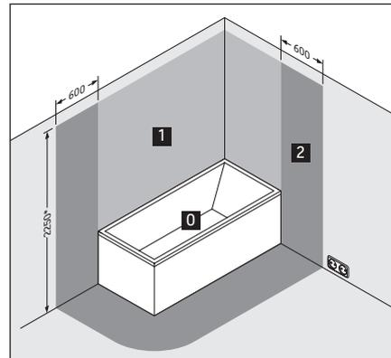
\* or the height of the highest shower head / water outlet that is permanently installed; depending on which is higher
